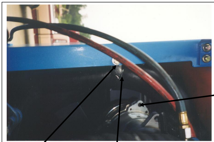
3/8" x 1" bolt Lower rad hosed support bracket
